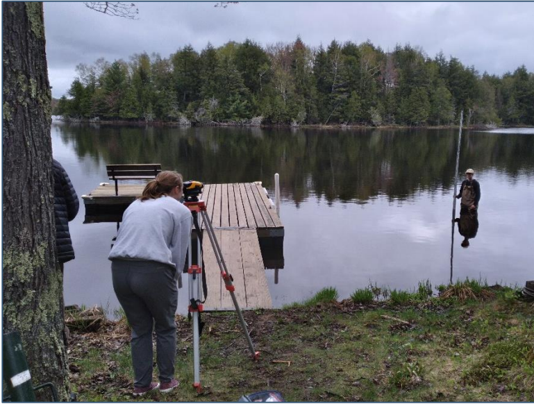
Figure 9 (Top): NLDC Staff installing lake level gauges as a part of our long-term lake level monitoring project.
